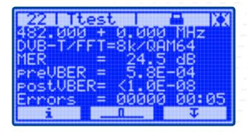
In this mode the screen displays the measured signal quality parameters of DVB-T or DVB-T2 channels in the form of a table. Users can change the display to view Channel info, ECHO or Constellation diagram.
