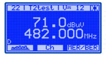
The IT-15T2 can measure signal levels of both analog and digital channels. For analog signals the meter will display the video carrier level, video frequency, C/N, and V/A ratio. For digital channels, the IT-15T2 measures the digital average channel power and displays the center frequency.
