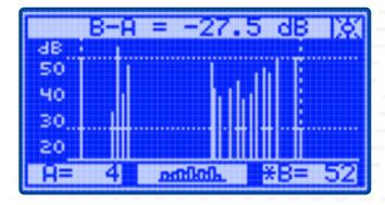
In this mode you will see the channels signal level as vertical bars and two dashed lines of ripple between two selected channels. The tilt function shows a graphical and numerical representation of the channel level, slope line between the peaks of selected channels with or without the specified frequency plan.
