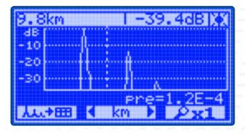
In this mode you will see the impulse response curve of DVB-T or DVB-T2 channels and also the basic signal quality parameters.
